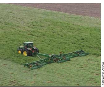
SFF, funded by the Howard G. Buffett Foundation, uses a 60-foot roller crimper to kill a cover crop in research designed to achieve standard corn yields using no synthetic fertilizer. This roller crimper is likely the widest in use in the world. It is designed to fold to less than 12 feet in width for transport so it can be used in a traditional farm operation.
