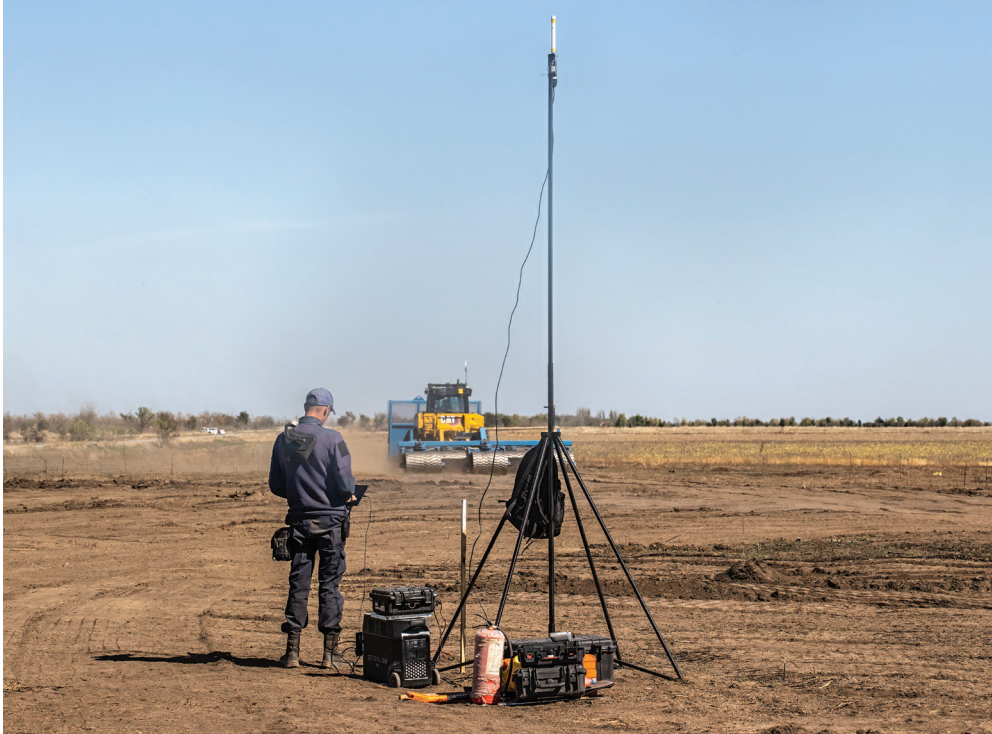
Above: A HALO mechanical operator oversees an autonomous bulldozer with a front and rear roller used in demining operations. Autonomy has the potential to significantly increase the efficiency of demining large agricultural fields.
